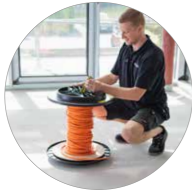
Place a CONTOUR wheel on the outside of the assembled cable drum. Now, switch the lever. This activates the inner tension care and the CONTOUR wheel is tightened to the drum.
